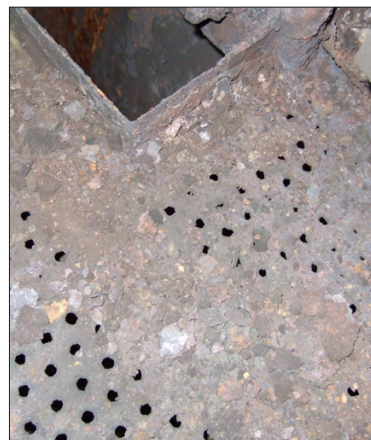
Figure 5 Scale fouling on sieve tray
