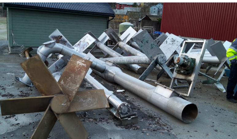
Great power savings could be achieved with Scaba hydrofoil high-efficiency impeller (below) versus pitch blade turbine (left).
